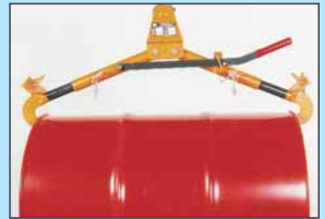
Engagement of barrel in horizontal position
