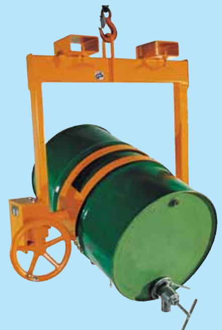
Turning gear: maintenance-free, self-locking
