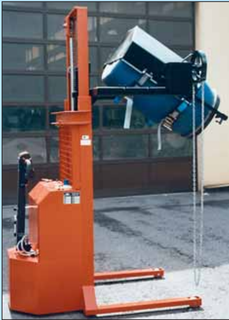
With electric travel-drive, electrical-hydraulic lifting and turning device manually operated.
