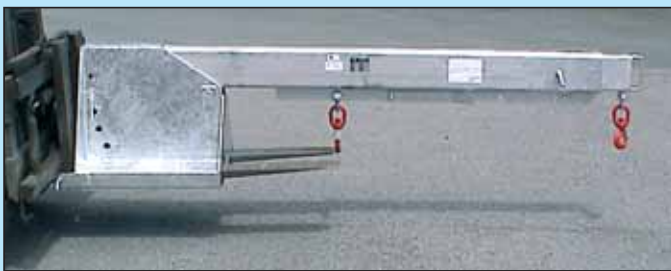
Crane jib 5 height settings, 6 length settings.
